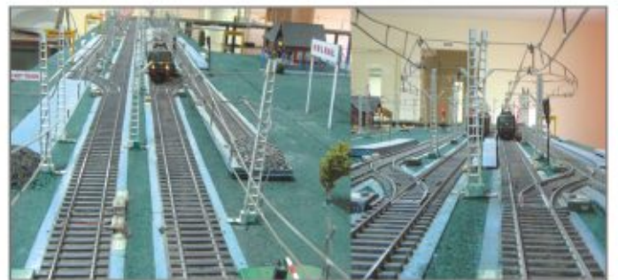
A functional test bench for Preliminary Evaluation of Railway Electronics Signaling Products at HBL Power Systems Limited
